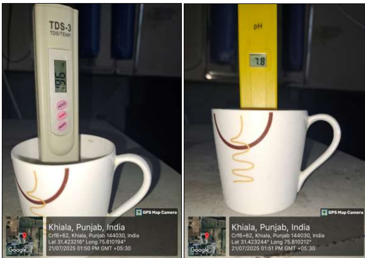
MEASURED PH VALUE AND TDS VALUE OF FILTERED DRINKING WATER
